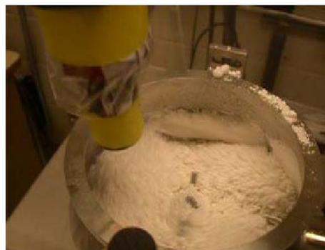
**Figure 1.** The non-contact probe of the *P<sup>h</sup>AT System*, covered by a temporary shield, monitoring material in situ in the granulation bowl.
