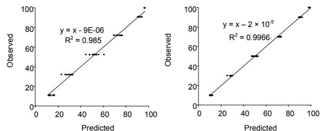
**Figure 2.** Calibration curves for theophylline obtained with (A) a standard system utilizing a ¼" IO and (B) the *P<sup>h</sup>AT System*.
